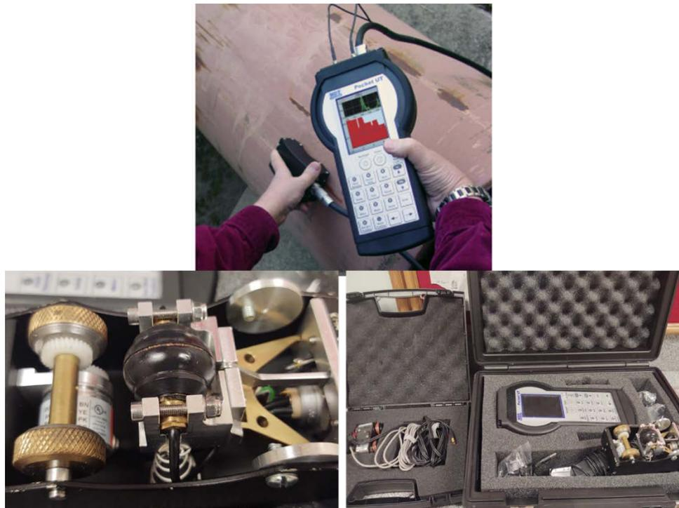
*Figure 49: Pocket UT hand-held scanner with remote pulser/receiver/display unit and roller probe and cables.*
