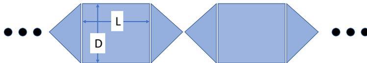
*Figure 6: The conceptual shape of the train-like robot module.*
