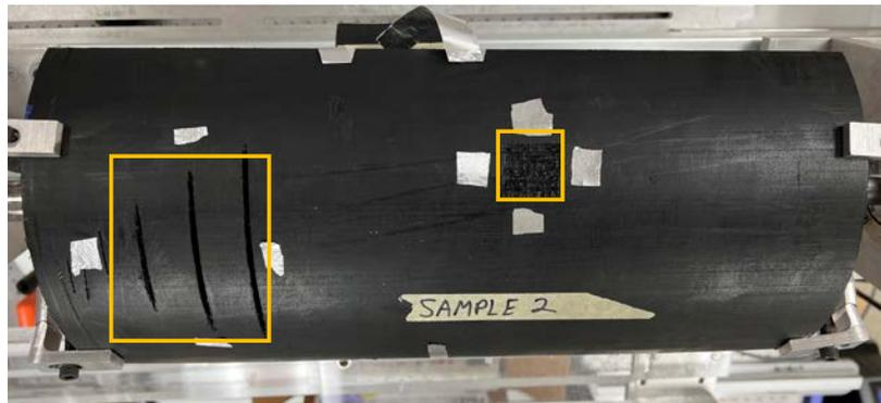
**Figure 14: Three slot cuts (left) and one square roughened area (right as enclosed) made on sample #2.**
