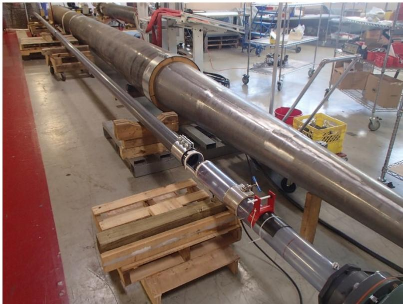
*Figure 3: Flow loop for testing of basic concept.*
