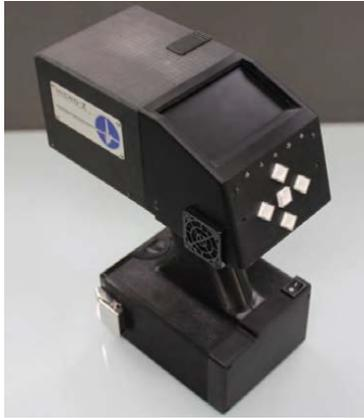
**Figure 30: Micro-Z: a handheld spectrometer as one of earliest miniaturized THz system [3].**
